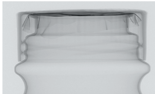
FINISH & CLOSURE WITH ALUMINIUM FOIL SEAL
