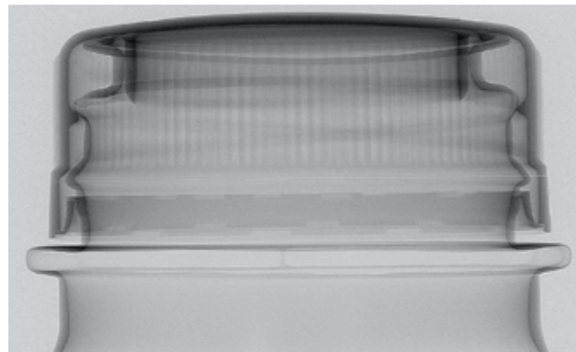
FINISH & CLOSURE WITH INTERNAL PLUG SEAL
